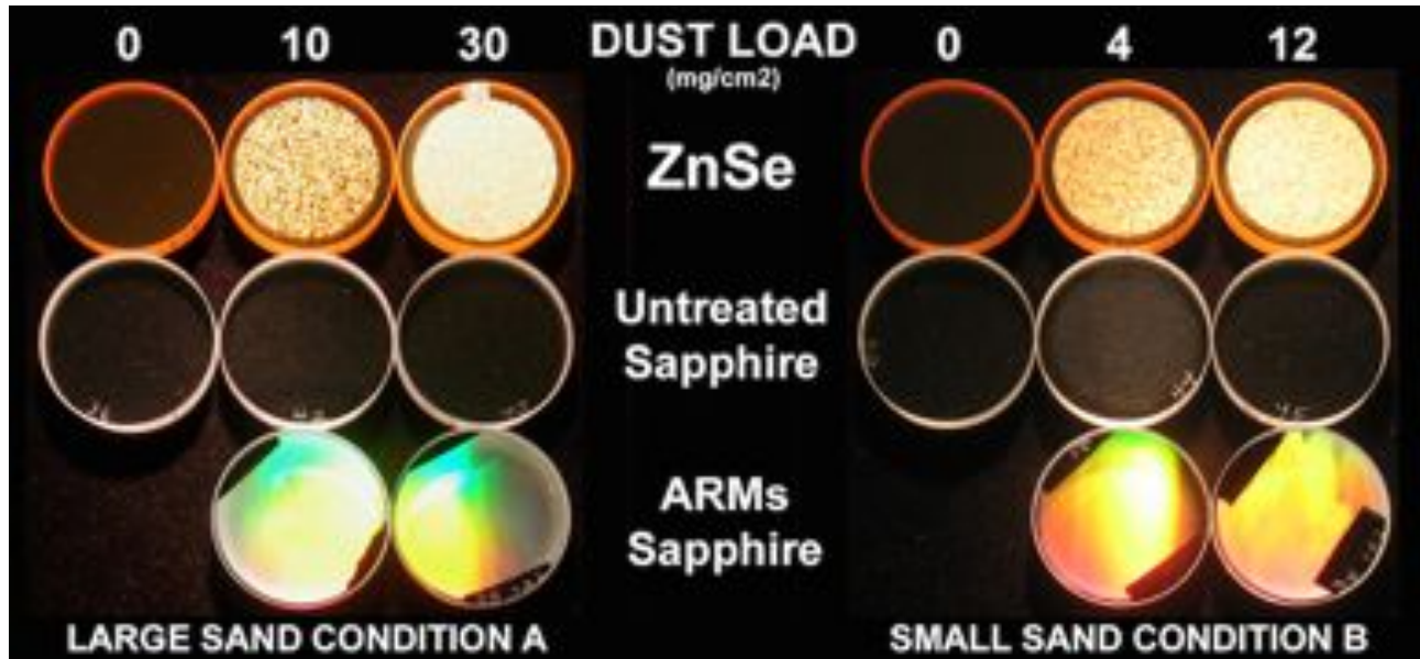
Figure 5: Sapphire and ZnSe windows after sand exposure in the UDRI particle erosion rig.
